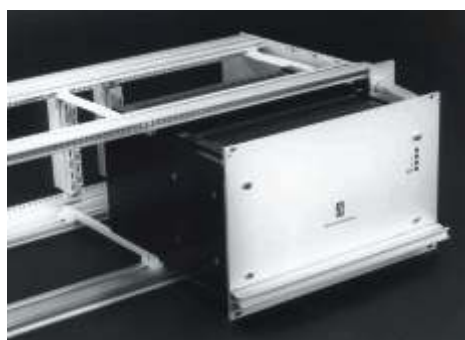
Eurorack mounting with front panel FP40
